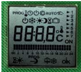
LCD 08019 TN Size: 46.5*44*2.0 mm Drive: 1/4 Duty; 1/3 Bias, 3V
