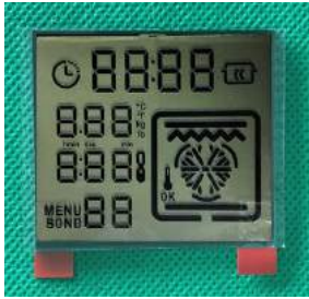
LCD 10020 HTN Size: 54*44*2.8 mm Drive: 1/4 Duty; 1/2 Bias, 5V
