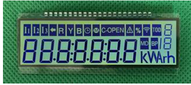
LCD 17039 Size: 66.0*25.7*2.8 mm Drive: 1/6 Duty; 1/3 Bias, 3V
