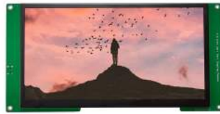
7.0" Serial port TFT display Resolution: 800*480 Size: 194.2*107.84*11 mm
