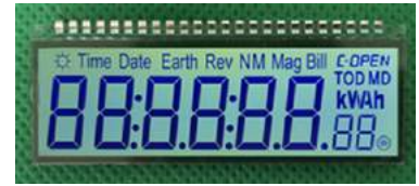
LCD 18008 Size: 54.5*19.5*2.8 mm Drive: 1/4 Duty; 1/3 Bias, 3.15V
