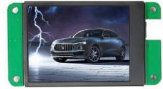
2.4" Serial port TFT display Resolution: 240*320 Size: 78.11*44.02*7.56 mm
