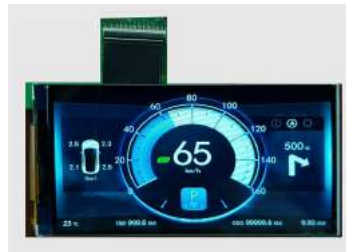
3.97" TFT for Motorcycle Resolution: 800*480 Size: 95.5*56.2*2.15mm
