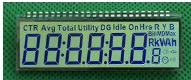
LCD 08030 Size: 54.5*19.5*2.8 mm Drive: 1/4 Duty; 1/3 Bias, 3V
