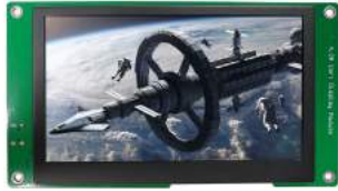
4.3" Serial port TFT display Resolution: 480*272 Size: 130.1*73.81*9.1 mm
