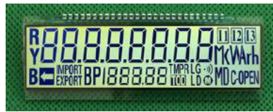
LCD 18015 Size: 79.7*26.2*2.8 mm Drive: 1/6 Duty; 1/3 Bias, 3V
