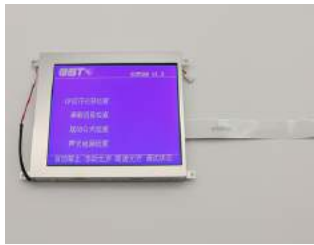
DG-32024002-V1 Resolution: 320*240 Size: 157.7*111.0*11.6 mm
