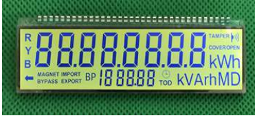
LCD 10002 Size: 79.7*23.7*2.8 mm Drive: 1/4 Duty, 1/3 Bias, 3V
