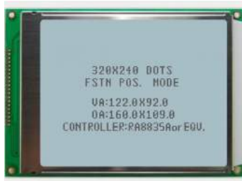
DG-32024001-V1 Resolution: 320*240 Size: 160.0*109.0*13.5mm
