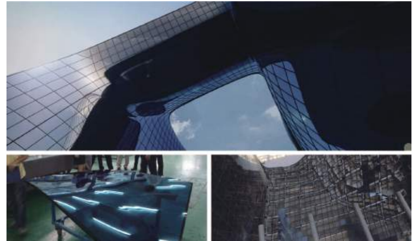
Project : Opus Configuration: 8mm Low – E+16A+6mm Clear glass+1.52mm PVB+6mm Clear Glass Location: Dubai
