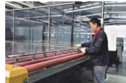
Tempered size inspection 钢化尺寸检验
