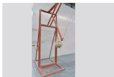
Tempered /Laminated shot-bag test 钢化/夹层霰弹袋实验
