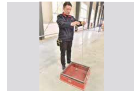
Tempered falling ball impact test 钢化落球冲击实验
