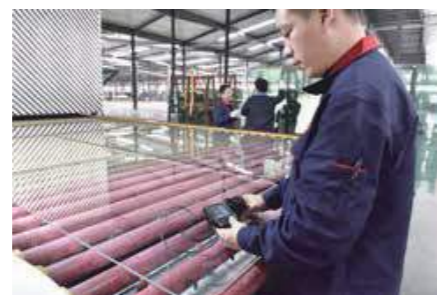
Tempered compression detection 钢化应力检测
