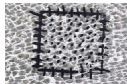
Tempered fragmentation detection 钢化碎片检测
