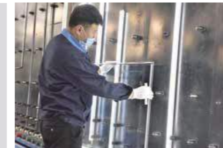
IGU make-up inspection 中空合片校验
