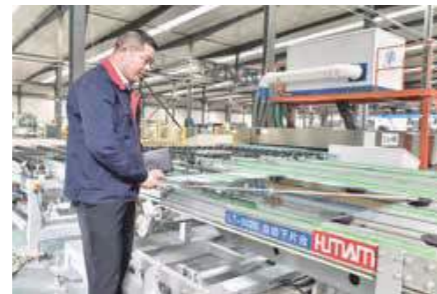
Cleaning appearance size verification 清洗外观尺寸校验
